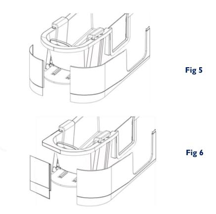
When a peninsula bath is being fitted the side panel without a door cutout must be fitted first. To do this correctly line up the panel with the bath shell (non door side), and firmly press forward on the top of the panel, engaging the panel top lip into the clips under the bath rim. Do not push too hard, as pushing too hard may detach the clips from the bath shell.
