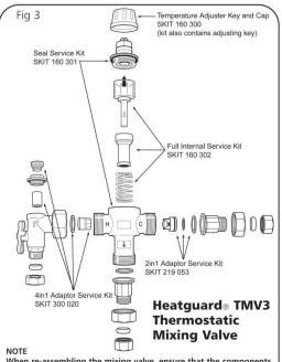
When re-assembling the mixing valve, ensure that the components are replaced in the correct order (as illustrated). Use only WRAS Approved silicon based waterproof grease.
